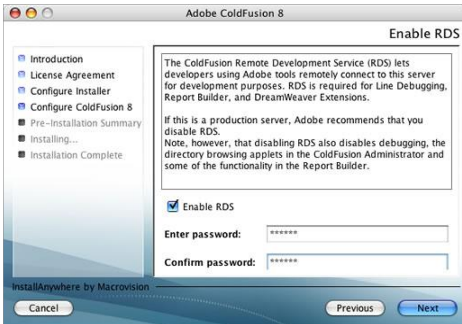
Figure 9. Enabling the RDS option before entering a password at the RDS Password screen (Macintosh).
